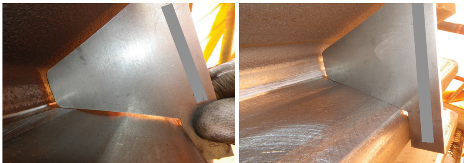
Figure 6. Profile deformation before intervention: 4.7 mm (left) and profile deformation after reprofiling by NOVEXA: accuracy 0.07 mm (right).
