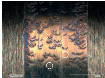
Fig. 5 Early detected mild damage with a 460 mm 2 /s market grease after 2 million cycles
